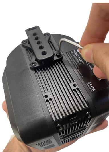
Lower the backpack handle and attach the scanner to the base of the antenna pole. Ensure that the bracket is fully inserted, and that the scanner is secure and does not move.
