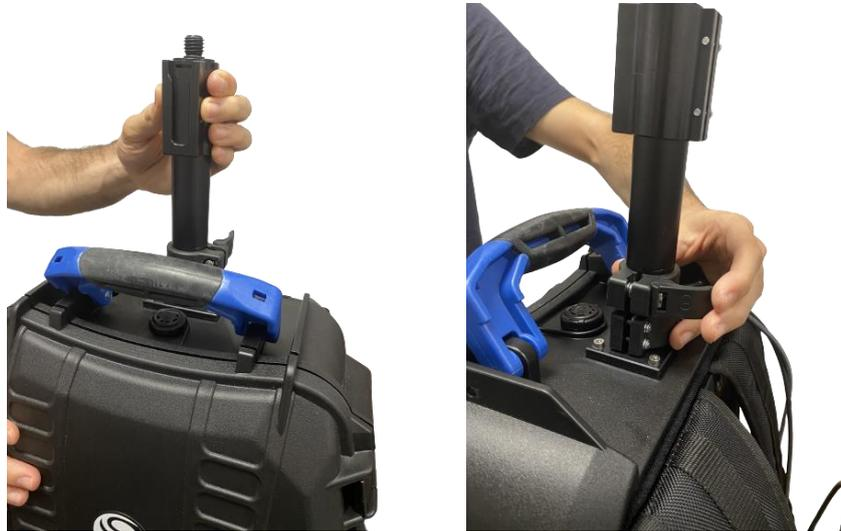
Screw the long part of the pole into the base.
