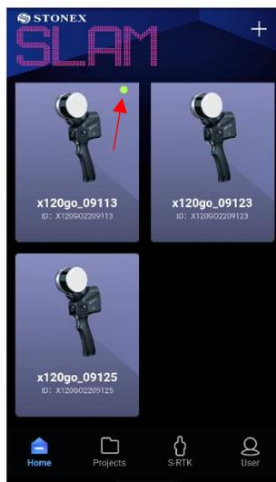
After successful connection, the equipment will be initialized. Click on **Start work** to start the scan.
