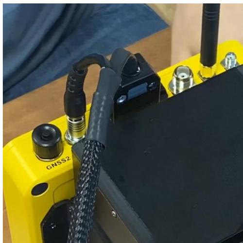
Slide the antenna pole into the antenna compartment, then run the antenna cable through it. Finally, install the geodetic antenna and connect one end of the cable to the antenna and the other to the SC600+.
