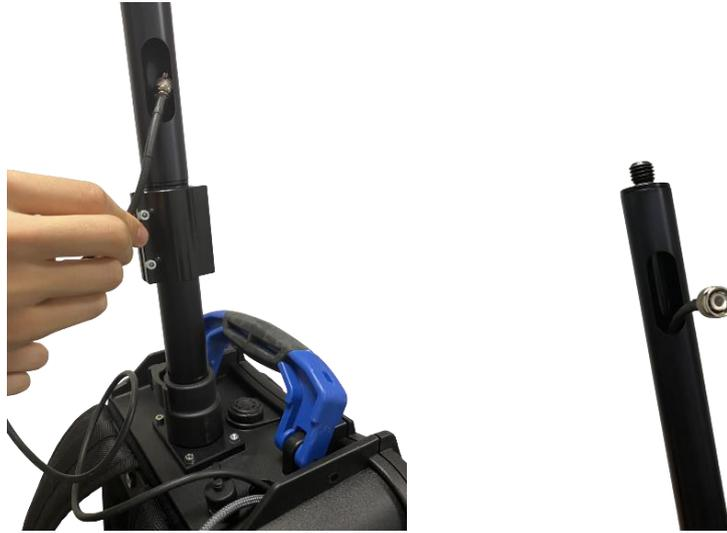
Screw the antenna SA85 into the upper part of the pole and secure it.
