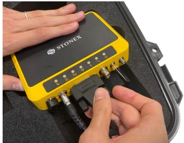
Connect the antenna cable to the GNSS1 socket and secure it. Pass the cable through the hole in the top of the backpack.
