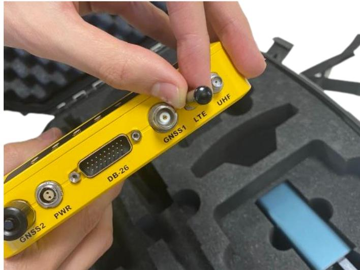
Place the instrument in the space above the battery and connect the 2-pin cable into the PWR socket (aligning the red dots) and the 26-pin cable into the DB-26 socket, taking care to secure it well.
