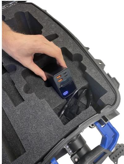
Plug one end of the cable into the power bank "In/out" port and the other into the scanner's type-c port. Pass the cable through the opening in the top of the backpack.
