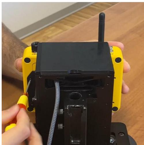
Install X 1 20 GO using the quick-release connector. Tighten the front screw placed under the scanner.
